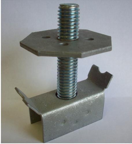
G-Clip™ model **GM-1/2”** is a galvanized carbon steel fastener used to fasten lightweight devices to 19-space bar grating. The GM-1/2” is designed to be used instead of J-bolts. It will withstand 1000 pounds of direct upward pull force.
