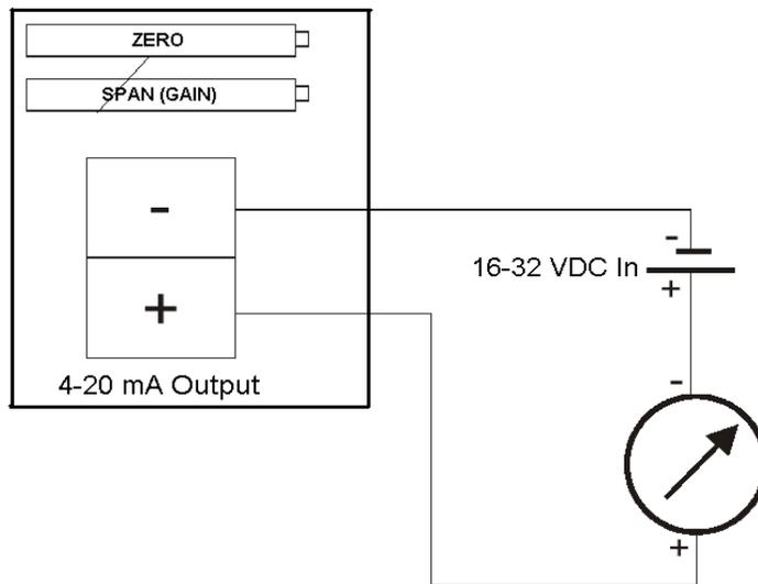
Type 2: Magnetostrictive sensor with 4-20 mA, 4-wire transmitter
