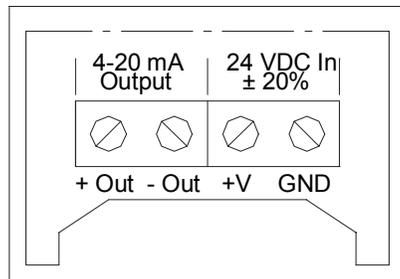
To minimize interference caused by electrical fields from other circuits, the low-voltage and signal cables should not be installed in the same conduit with high voltage cables.
