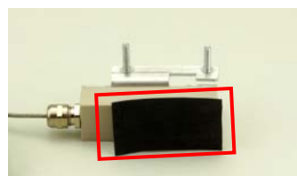
Picture 6 Using acoustic coupling foil
