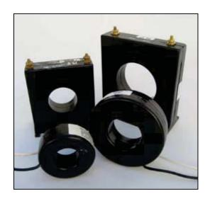
**5Amp Secondary Current Transformers** offer a compact, cost-effective means of measuring primary current and providing 0–5A secondary output proportional to the primary current being sensed. Available in solid-core or split-core enclosures.
