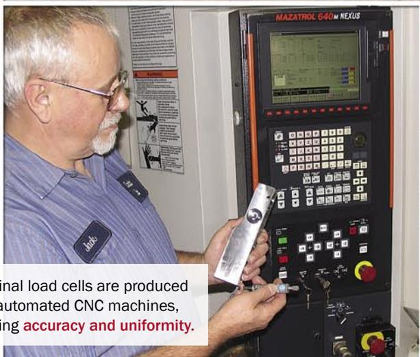
Cardinal load cells are produced by automated CNC machines, assuring **accuracy and uniformity**.
