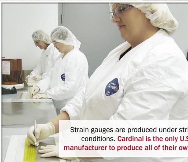
Strain gauges are produced under strict clean room conditions. **Cardinal is the only U.S. load cell manufacturer to produce all of their own strain gauges.**
