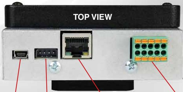
**Mini USB-B** **Remote Display** **Ethernet** **Remote I/O**
