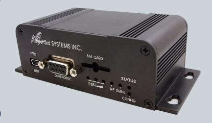
The IPn3G provides a communications hub bringing together serial (RS232 and RS485), Ethernet, and USB channels into a single box. It provides secure, reliable communications where needed. It features flexible maintenance utilities, secure Firewall, Access Control Lists, IPSec / VPN and Network Management Utilities.
